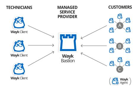
In this example, an MSP deploys a single **Wayk Bastion** server in a network location that is accessible to all of its customers. All of the machines that are centrally managed in **Wayk Bastion** have **Wayk Agent** installed on them. As a result, technicians can use **Wayk Client** to connect to machines with **Wayk Agent** through **Wayk Bastion**.
